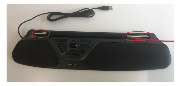
Finish off by cleaning the wrist rest and buttons with wet wipes, removing dust and grease on the surface of the RollerMouse.
